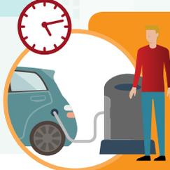
**Jim** arrives home from work, plugs in his EV and sets the charge priority to high which guarantees him a full charge by the morning. He's off on holiday tomorrow and has a long drive in the morning so needs the car battery to be at full capacity. The Hub detects the car being plugged in and removes the offer of flexibility from the community energy scheme.
