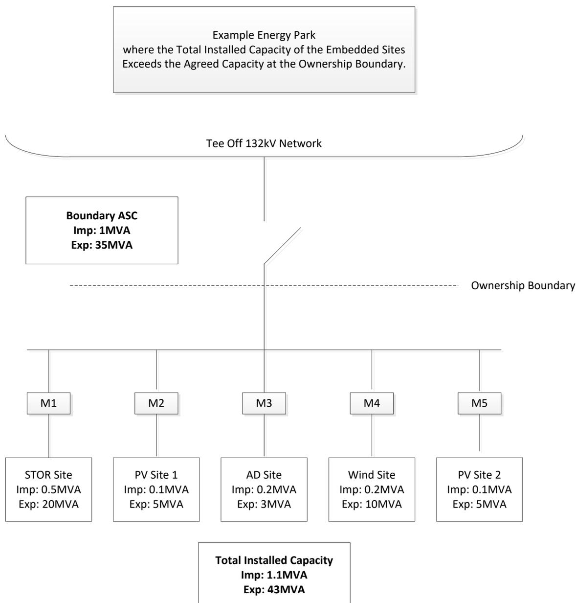
In the above example of an “Energy Park” the DNO has given the connection agreement holder 5 pairs of import/export MPANs for use with the 5 embedded meters shown<sup>1</sup>. Each of the 10 MPANs has been allocated a site-specific LLFC to enable trading using the “Fully Settled Metering Option” as described in the Elexon Guidance note for Licence Exempt Networks.
